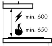
**IMPORTANT** These dimensions are a guide only. All measurements are in millimetres (mm). For complete installation instructions, refer to the manual provided with product.
