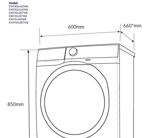
\*Add 20mm for the hose protrusion at the back.
