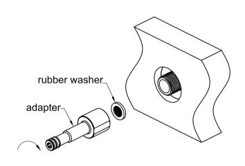
3. Slide plate, washer and spout onto adapter successively, then screw grub screw into spout with allen key firmly.
