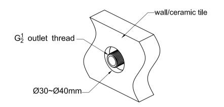
2. Screw the  $G_2^1$  spout adapter on the outlet thread, and ensure there is rubber washer inside, as shown in the figure.
