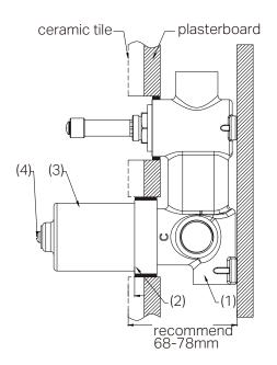
4. When the installation depth is 68-70mm, make the protective sleeve (2) 2-4mm from ceramic tile surface to body.
