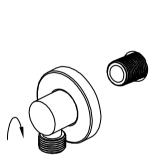
Screw elbow body on to outlet.
