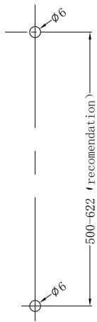
4. Drill two  $\Phi$ 6mm holes according to above picture.
