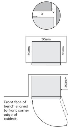
If you have a cupboard above the refrigerator with a rear gap of less than 100mm (Y), recommended minimum clearance at the top of the refrigerator increases from 30mm to 70mm (X).
