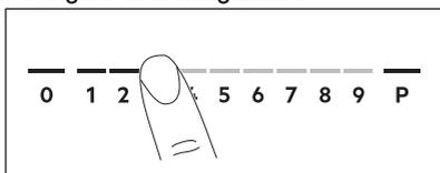
Once you place a pot on the cooking zone and set the heat setting, it remains the same for 50 seconds after you remove the pot. The control bar blinks for the second half of that time. If you place the pot on the cooking zone again within this time, the heat setting reactivates. Otherwise the cooking zone deactivates.
