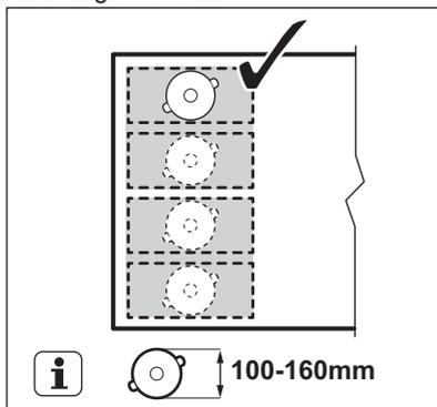
Place the cookware with the bottom diameter larger than 160 mm centrally between two sections.
