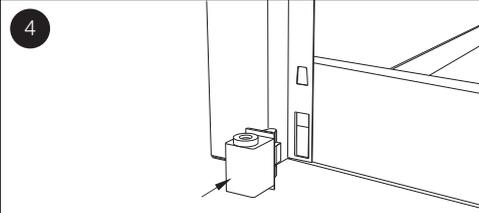
Press fit the Hinge Base (5) into the corresponding hole in the side panel on the side you would like the door to hinge.
