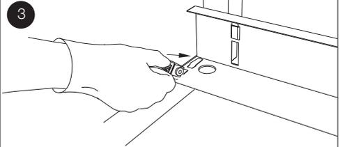
Using the Hinge Base (5) as an assembly aid flatten the 8 base tabs to lock the panels together.
