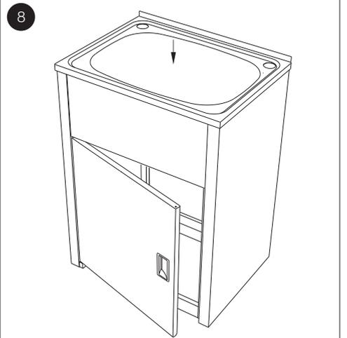
Install Waste and Bypass fittings supplied with Tub. Position Tub (8) on top of the Cabinet Assembly.
