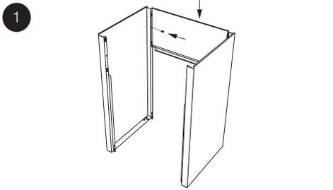
Slide one Front/Rear Head Panel (2) onto Side Panels (1) and snap Panel Fixing Clips (3) into place.
