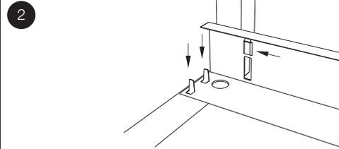
Slide both Kick Panels (4) (Front and Rear) onto the 3 tabs in the bottom corners of the side panels.
