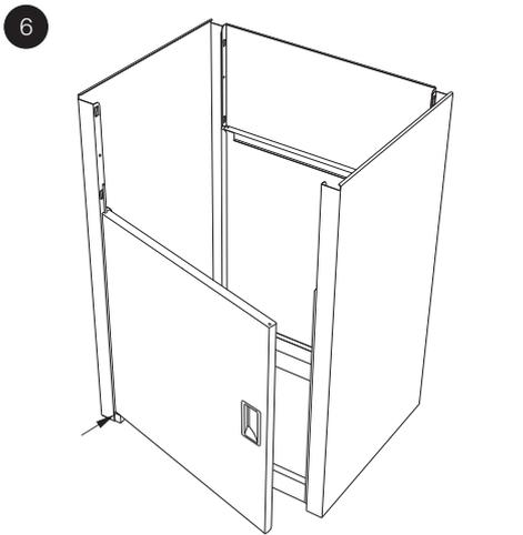
Align and insert the Door Assembly (7) with the corresponding holes in the Hinge Base (5).
