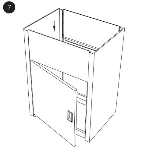
Align the second Front/Rear Head Panel (2) with the Side Panels (1) and slide over the Door Hinge Rod (6). Snap the remaining two Panel Fixing Clips (3) into position.
