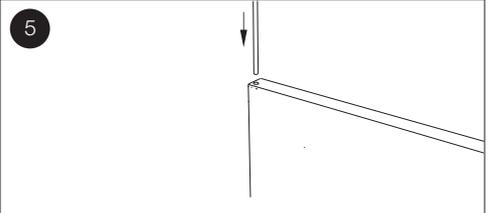
Insert the Hinge Rod (6) through the holes on the Door Assembly (7).
