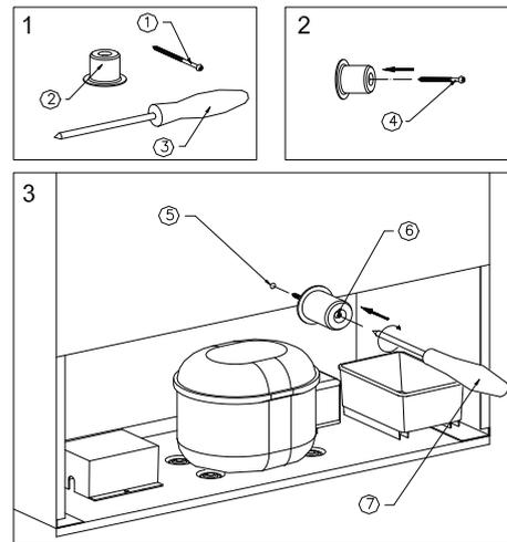
**IMPORTANT - THIS SPACER MUST BE ATTACHED TO THE UNIT BEFORE THE INSTALLATION, FOR VENTILATION PURPOSE.**
