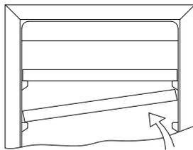
1. Open the door to a 90 degree angle, take out the 2 screws from door axis, remove the door, Remove the Door axis.
