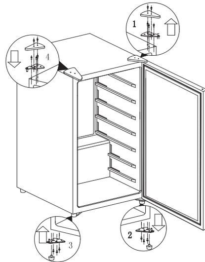
1. Unscrew and remove the decorative cover. While holding the door firmly, loosen and remove the top hinge, lift up and remove the door.
