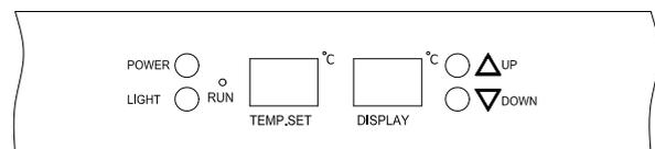
To modify the pre-set temperature of VWS035 models Adjust the desired cooling temperature by pressing the UP or DOWN buttons. Each depression of the buttons will scroll through the available temperature settings in increase or decrease of 1 degree Celsius.
